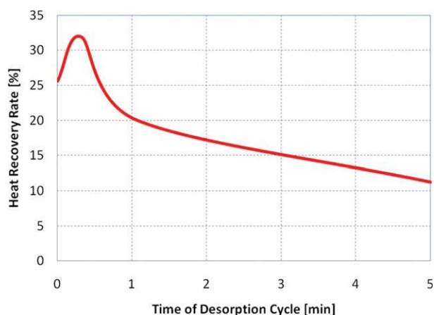
Figure 12. Heat recovery rate during the desorption cycle.
